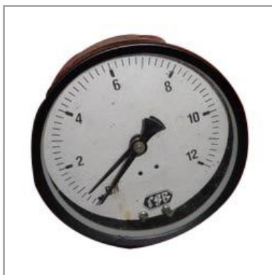
Differential Pressure Gauge
